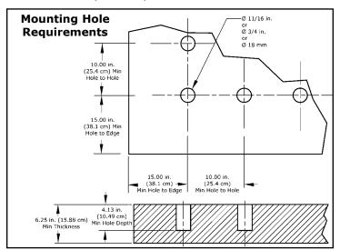
**Standards and Warranty** Reliability that saves you worry, time and money. Complies with OSHA and ANSI requirements including ASTM E488 Standard Test Methods for Strength of Anchors. The reputation of DBI-SALA stands behind every one of our products supported by a two year warranty on parts and workmanship.
