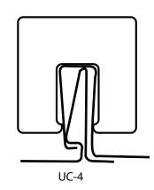
There are a few profiles which are marginal. One example is Copper Sales UC-4 (at left). The clamp will fit over this profile, but must be slipped on from the end and then carefully moved to its desired location. Another example is Berridge "Cee Lock." The S-5-U will fit this profile, but it may have to be forced down until it snaps over the seam profiling (far left).
